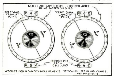
Fig. 3, Dial calibrations—A scales for capacities and 8 scales for inductances.
